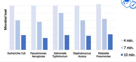
Up-to log6 microbial reduction with a 10 minutes treatment, at 3.5 mt from target Suface
