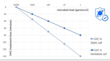
Up-to 99,99% microbial reduction on food surface inside a Ventilated Storage Cell, in 80 minutes.
