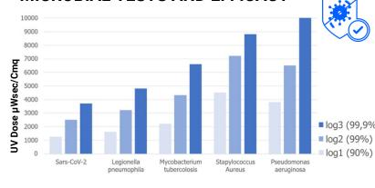
Up-to log3 microbial reduction on Airflow, Coils and HVAC surfaces, 24 hours a day.
